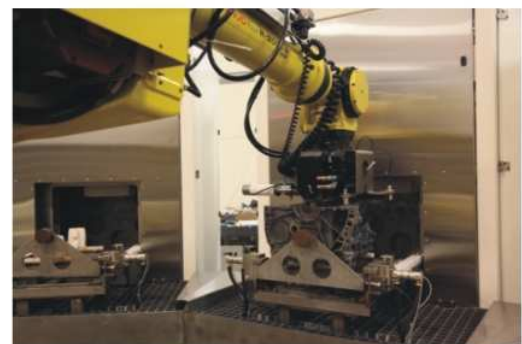
Godfrey & Wing's Fully Automated High Speed Single Piece Flow Impregnation System. Cycle time: 60 seconds.
