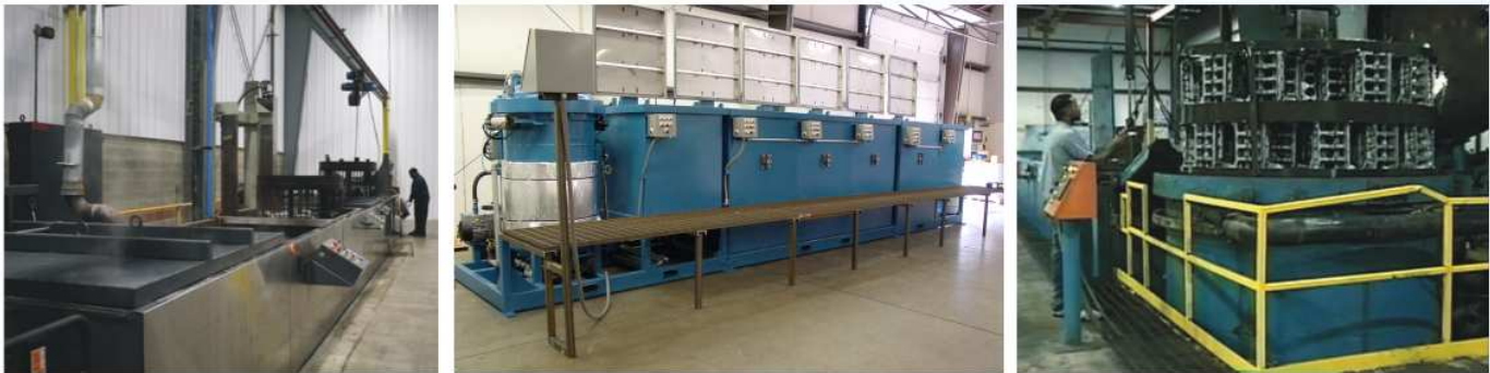
Godfrey & Wing's Standard Top Load Batch Systems from 14" to 60" in diameter. Cycle time: 30 minutes.
