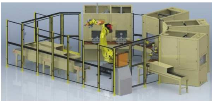
Godfrey & Wing's Fully Automated High Speed Single Piece Flow Impregnation System. Cycle time: 60 seconds.
